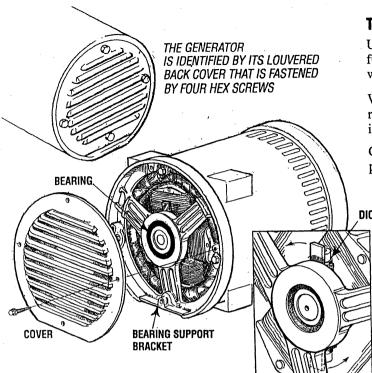
Testing the generator can be accomplished without removing the bearing support bracket. Simply turn the armature to allow access for the testing as shown.
