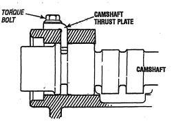
3. Measure the end play of the camshaft by inserting a feeler gauge in the gap between the rear of the thrust plate and the new front camshaft journal.
