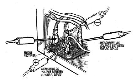
Normal DC voltage running out of the rectifier (in volts DC) is measured across the two DC connections of the bridge rectifier, that is + and - as illustrated.
