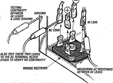
**TESTING THE BRIDGE RECTIFIER** (meter used - FLUKE multimeter)
