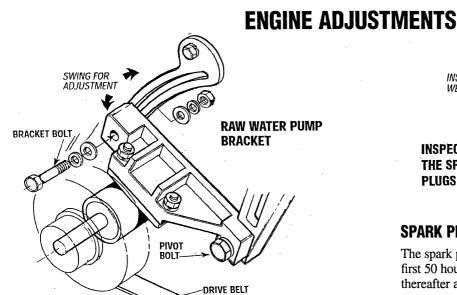
The generators have two drive belts, one drives the governor and alternator and the other drives the raw water pump. The drive belts are properly adjusted if it can be deflected no less than 3/8 inch (10mm) and no more than 1/2 inch (12mm) as the belt is depressed with the thumb at the midpoint between the two pulleys on the longest span of the belt.
