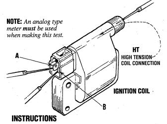
Unplug the electrical connections from the coil carefully noting the position of the two electrical connections  $\bf A$  and  $\bf B$  as they must be reconnected in the exact same position.
