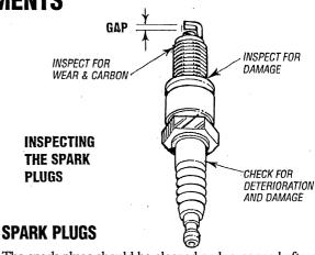
The spark plugs should be cleaned and re-gapped after the first 50 hour break-in period, then inspected every 250 hours thereafter and replaced as needed.
