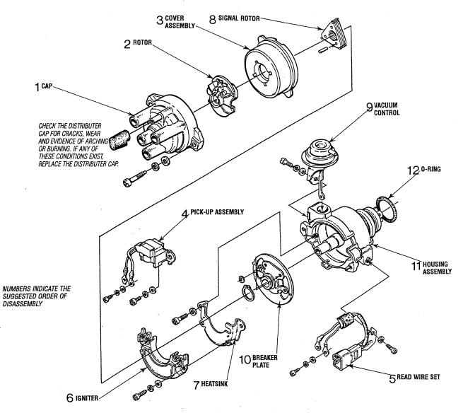
**NOTE:** When engaging the Distributer Drive into the Camshaft match the markings for correct engagement.
