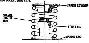
Use the valve spring compressor to compress the valve springs. With the valve spring compressed, remove the
