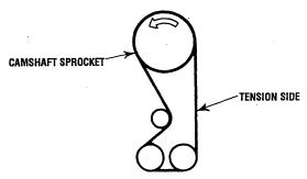
7. Loosen the temperorarily tightened tensioner nut on the water pump side 1 or 2 turns, and tension the belt making use of the spring force.
