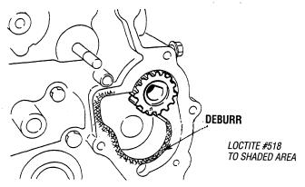
**NOTE:** Deburr this edge area as shown. Clean off all metal from the deburring process and clean with a cleaning agent. Wipe dry with a clean cloth and use compressed air to blow dry, the block surface and oil pump cover must be clean and free of oil.
