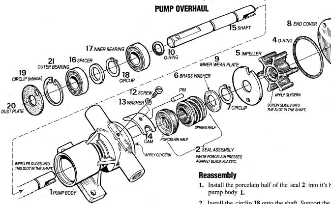
The pump when removed from the engine, will have hose attachment nipples threaded into its inlet and outlet ports along with the drive pulley attached to the shaft of the pump. In most cases the hose nipples can be left in place. Note their positioning. Remove the drive pulley.
