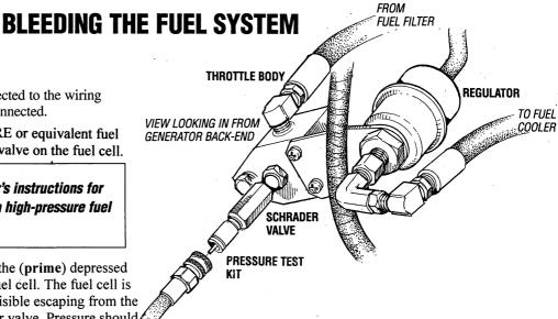
7. Repeat step 3, after attaching the pressure gauge set to the Schrader valve on the throttle body. The pressure should be 40 psi after purging all the air.
