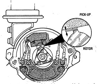
Adjust the point gap of the pick-up assembly between the rotor and the pick-up.
