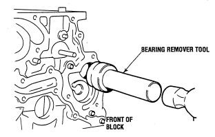
Use the same tool and drive the counterbalance shaft rear bearing from the cylinder block.
