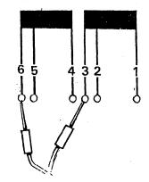
TEST EACH OF THE WINDING LEADS INDIVIDUALLY AS SHOWN
