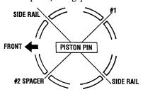
Insert the piston and connecting rod assembly into the cylinder, working from the arrow mark on the piston top toward the camshaft sprocket side.
