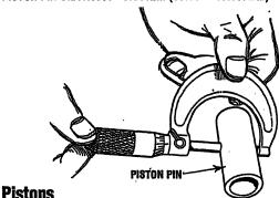
Check the piston surfaces for wear, seizure, cracks and streaking. If any damage is evident, replace the piston. Inspect the oil return hole in the oil ring groove and the oil hole in the piston boss. Clean the piston if these are clogged. Check the piston pin hole for signs of seizure or damage. Replace the piston if damage is evident. Measure the piston diameter at 90° (perpendicular) to the pin bore axis.
