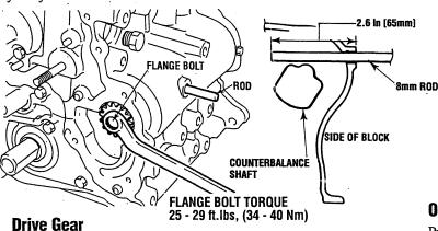
Align the timing marks and install the oil pump drive gear to the cylinder block.
