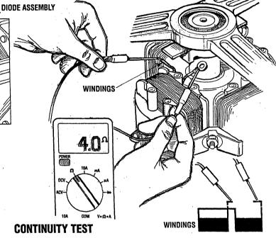
Check that no continuity exists between either of the winding leads and the generator shaft. If continuity is found, there is a short in the windings.
