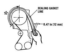
11. Pull out the rod from the plug hole on the left surface of the cylinder block and apply the specified sealant. Then tighten the plug to the specified torque.
